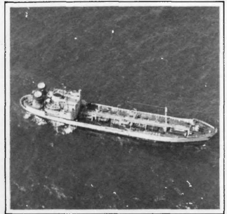
Dutch ship Vulcanus has two incinerators at the stern (left).
