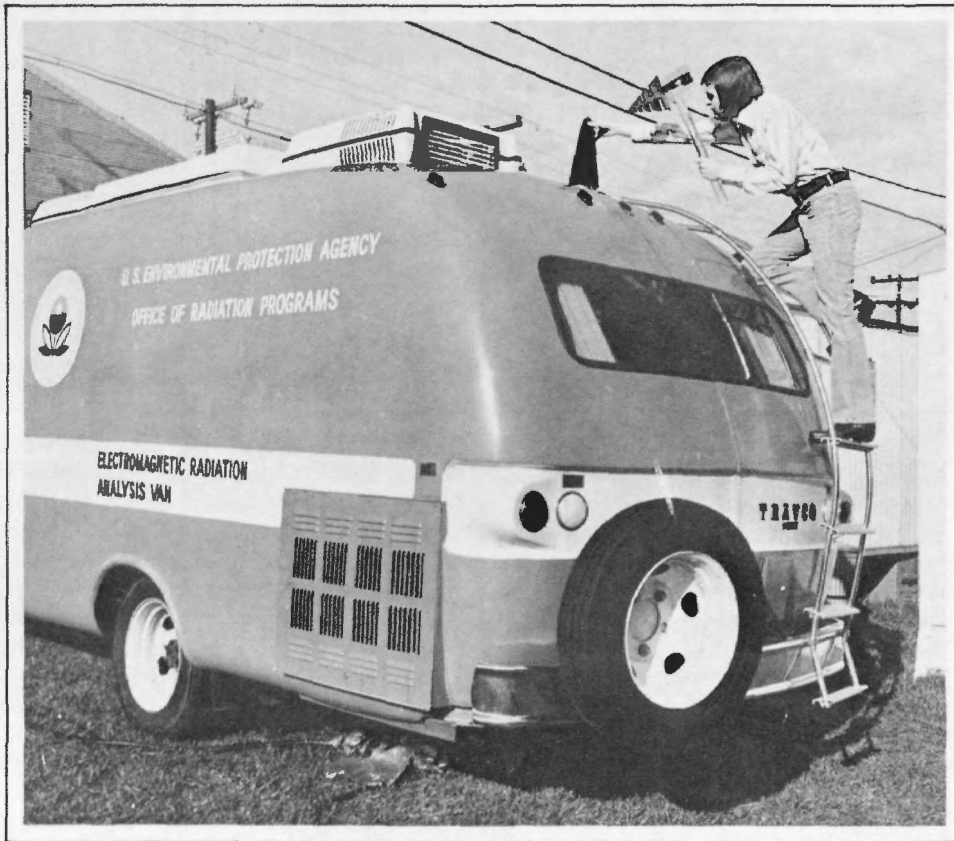
John Nelson climbs radiation analysis van to put microwave antenna on the traveling lab's mast. A pneumatic mechanism can lift the mast 10 meters, the better to detect and record electromagnetic fields.
